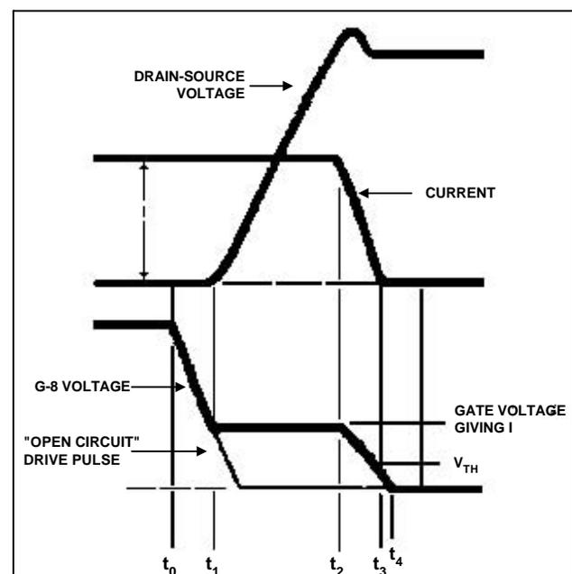
Figure 7 shows theoretical waveforms for two parallel connected HEXFET Power MOSFETs with their gates connected directly together. For purposes of discussion, the source inductance is assumed to be zero. At  $t_1$ , the gate voltage reaches the point at which HEXFET Power MOSFET B can no longer sustain its drain current.
