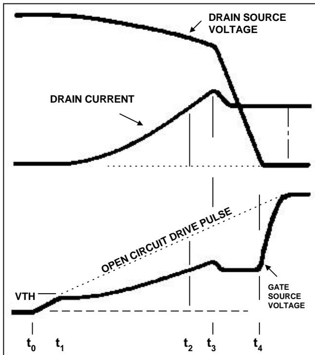
The problem will be introduced by considering the switching waveforms for a typical clamped inductive load. Figure 4 shows waveforms of drain current, drain-to-source voltage, and gate voltage during the turn-ON interval. For reasons of clarity we have shown the applied drive pulse increasing at a relatively slow rate.
