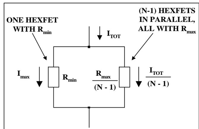
**Figure 3.** Simplified Equivalent Circuit for Estimating Worst Case Steady-State Current Unbalance
