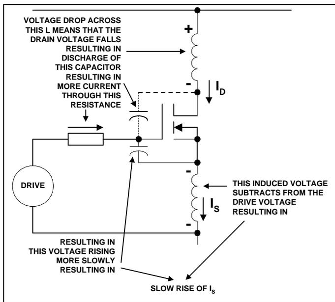
**Figure 5.** Diagrammatic Representation of Effects When Switching-ON
